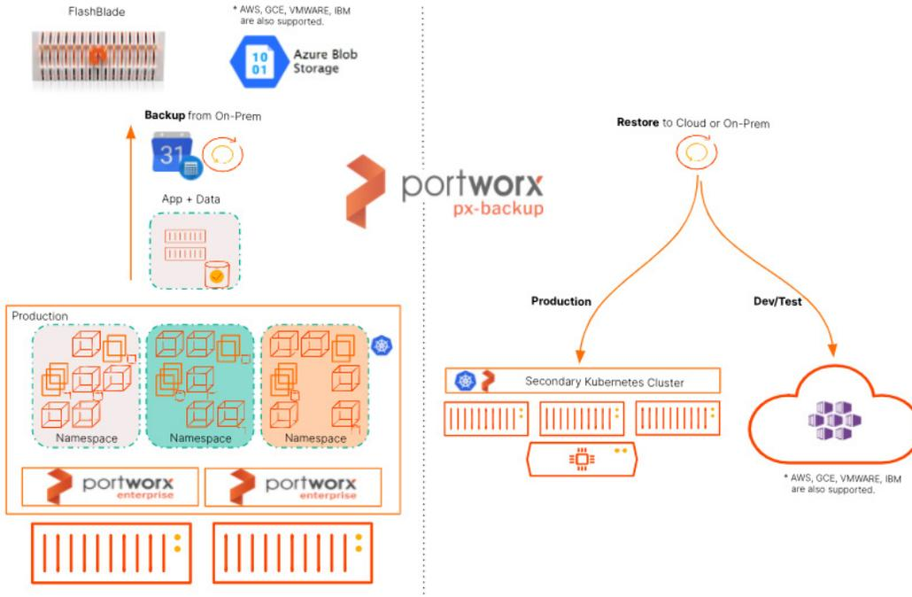
Figure 20. Using PX-Backup to create on-prem and cloud backups.
