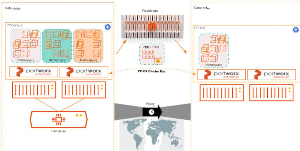
Figure 21. PX-DR (Asynchronous DR) On-prem to On-Prem.
